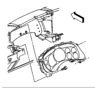
2 Remove the screws that retain the I/P cluster to the I/P assembly.
